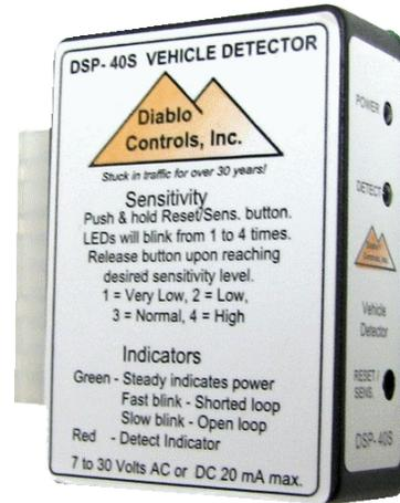
**Loop Failure** - The green power indicator flashes slowly if the loop circuit is open and quickly if the loop circuit is shorted. This detector will output a "Detect" for either of these loop failed conditions.
